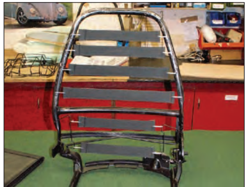
Replacing the webbing
